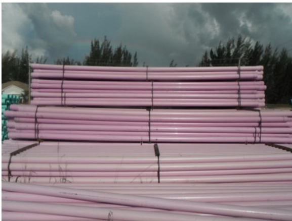
Irrigation Pipes (Purple Color Pipes)
